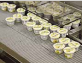
MASS LOW BACK PRESSURE ACCUMULATION TO SINGLE ROW ON STAINLESS STEEL FRAME
