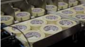
PATTERN FORMATION FOR ROBOTIC CASE PACKER
