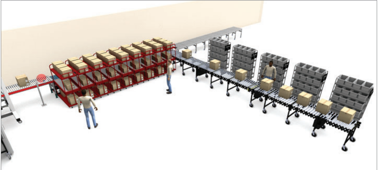
CASI-SORT distributes complete packages to WING CARTS and break-packs (eaches) to AGILITY Powered Flexible Conveyor.
